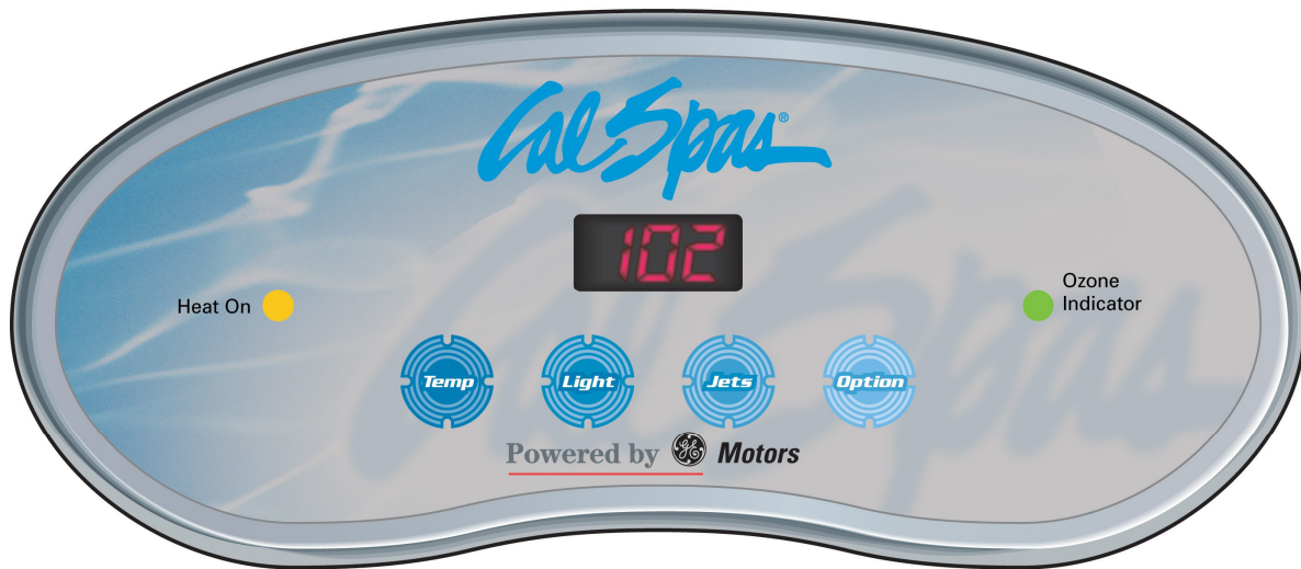
Figure 6. 6000 and 6100 Electronic Control Panel
