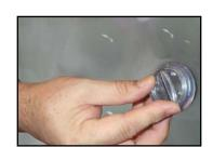
Step 10. Place the chrome ring cap back on and turn clockwise to tighten it down.
