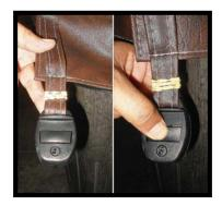
With the straps pulled taut (but not overly tight), lightly drill the location for screw placement. Gently drill 3 holes - one for each screw slot in the lock. (If you do not have a low torque drill, use the lowest torque setting on the drill you have.) DO NOT drill all the way in but instead just make a guide for starters.
